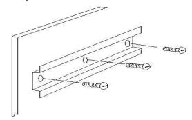
A : Fixing of Raceways
