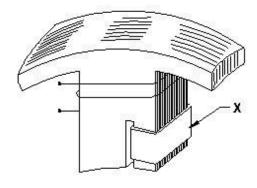
A : Main coilB : Shading coil
