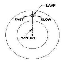
A : Indicating the fast directionB : Indicating the slow directionC : Visible at its central position
